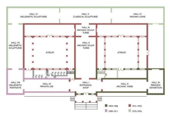
**Fig. 4.** Plan showing the construction stages of the Museum of Delos. **Source:** Hadjidakis 2003: 123.
